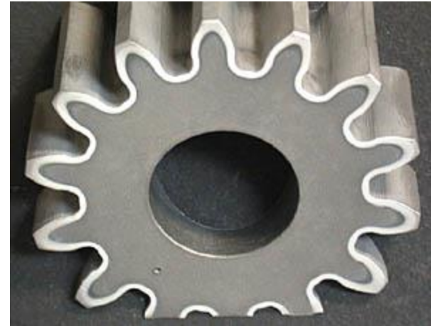
A 6150 spur gear profile hardened using single-frequency single-shot technique
