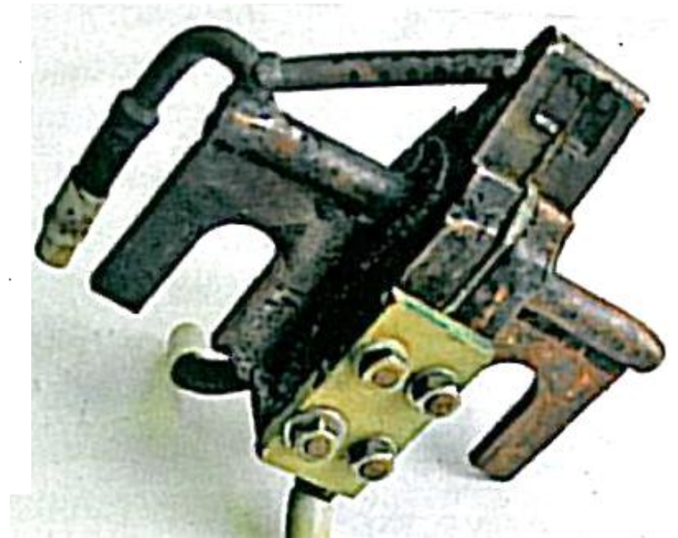
Used inductor for large gear hardening
