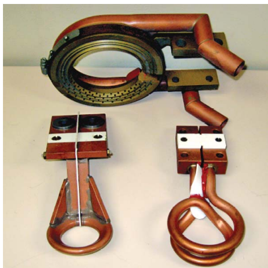
Fig. 1. Typical induction-scan hardening inductors and quench ring
