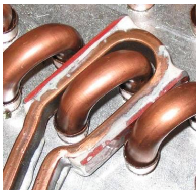
Figure 3. Brazing of reverse bent
