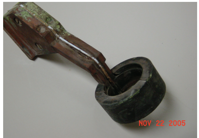
Figure 7: An image of the coil developed through prototyping, after producing over 170,000 parts
