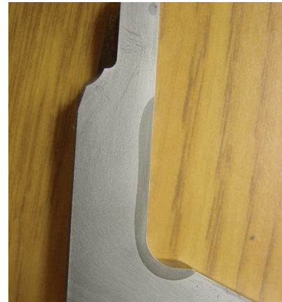
Figure 6: An image of a cut section of the wheel hub, showing the desired hardness pattern
