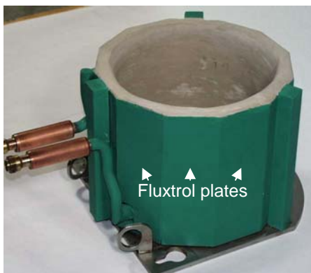
Fig. 5: Shielding of a melting inductor for glove box environment: left – final design; right – computer simulation
