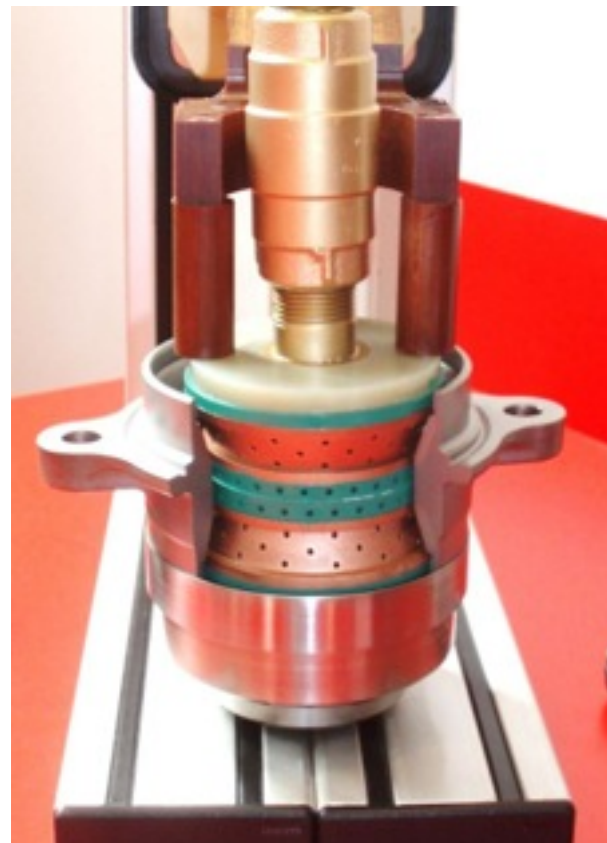
Internal coil with Fluxtrol controller (green)
