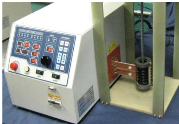
Figure 2. The entire testing system using the solenoidal coil with a field probe inside
