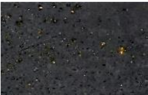
Figure 4. Close up of corrosion on Fluxtrol 100 sample having additional surface treatment coated with B material. after 168 hours of humidity testing.
