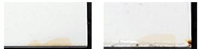
Figure 6. Close up of corrosion on Fluxtrol A with additional surface preparation (left) and without (right) after 168 hours of humidity testing with Coating C applied.
