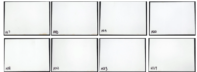
Figure 5. Coating C samples after 168 hours of humidity testing.
