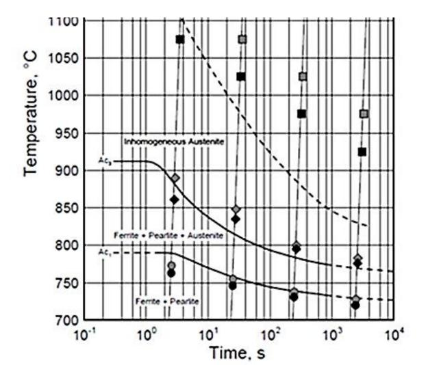
Changes in the microstructure of a Ck 45 (1045) steel with heating rate and peak temperature.
