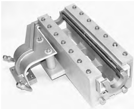
Fig. 3 Single-shot induction heat treating application
