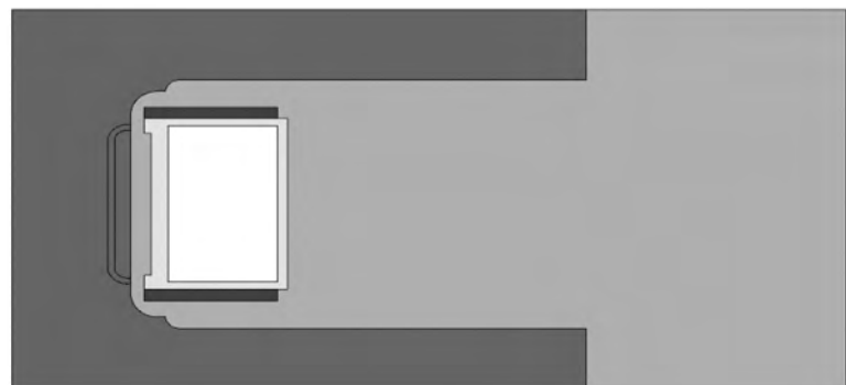
Fig. 16 Nonrotational inductor cross section used for simulation
