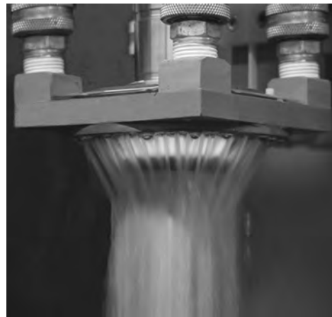
Fig. 6 Machined integral quench scanning inductor with magnetic flux concentrator
