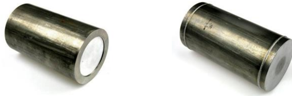
Figure 2: Steel-aluminum bimaterial billet where an aluminum core is inserted into a steel tube on the left and two steel end caps are welded to the tube to complete the assembly on the right.
