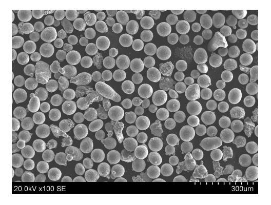
Typical titanium aluminide power. It is typical for some of the particles to be broken.
