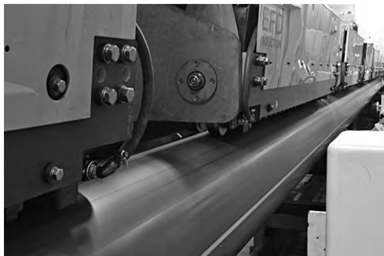
Fig. 25 Seam annealer for tube-welding line. Courtesy of EFD Induction
