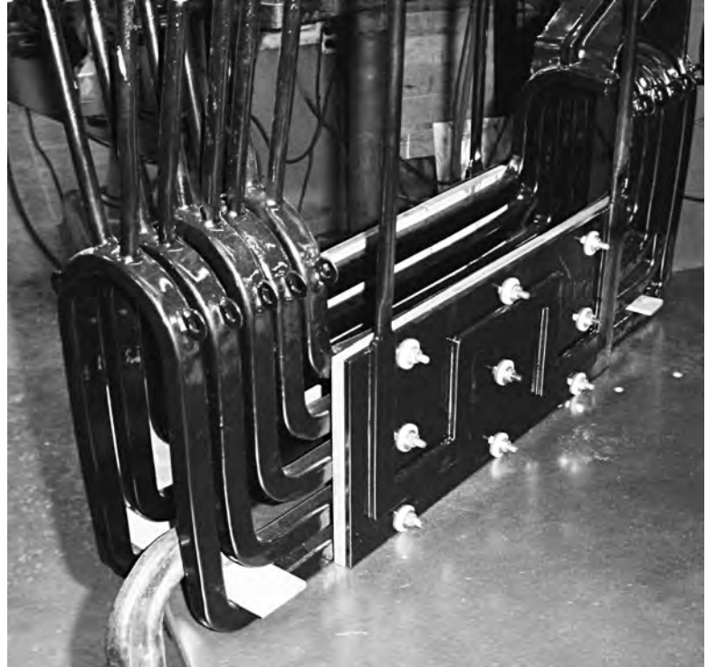
Fig. 20 Continuous bar-end heater with magnetic flux concentrator. Courtesy of Fluxtrol, Inc.
