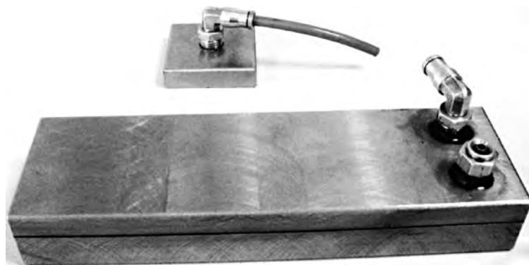
Fig. 11 Soft magnetic composite material with channels for direct water cooling. Source: Ref 4
