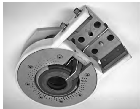
Fig. 27 Two-turn scan hardening coil with magnetic flux controllers used for axle scan hardening. Source: Ref 4
