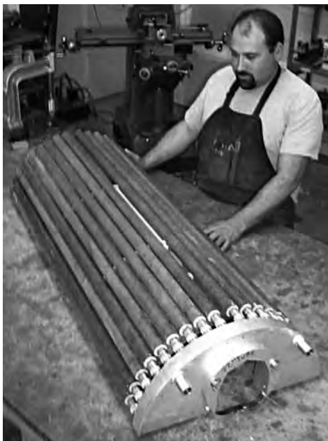
Fig. 23 Cluster impeder (multiple impeders assembled together) for large diameter pipe welding. Courtesy of Electronic Heating Equipment, Inc.
