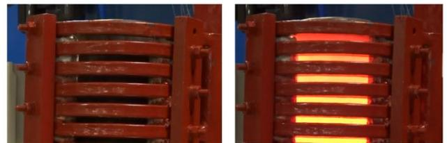
Figure 14. 1/4" wall bimetal billet before and several seconds after a 4 second heat pulse at 400 – 500 kW, 10 kHz.
