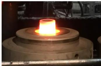
*Figure 15. 1/2" wall bimetal billet before 2 seconds after a 26 second, two stage heating cycle*
