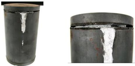
Figure 5. Cracking and leaking of the Al after heating to 600C, 0.5" billet
