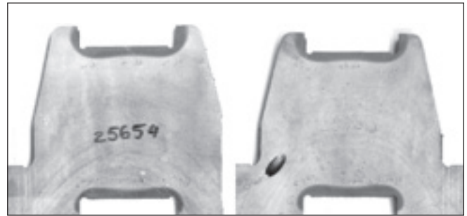
Fig. 4. Heat-treatment pattern for a fillet-hardened crankshaft with laminations (left) and Fluxtrol A (right)
