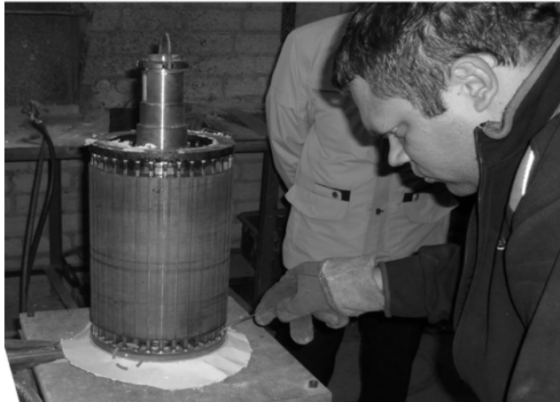
Fig. 3. Final stage of the brazing. Spot on a ring – a point of the pyrometer laser pointing
