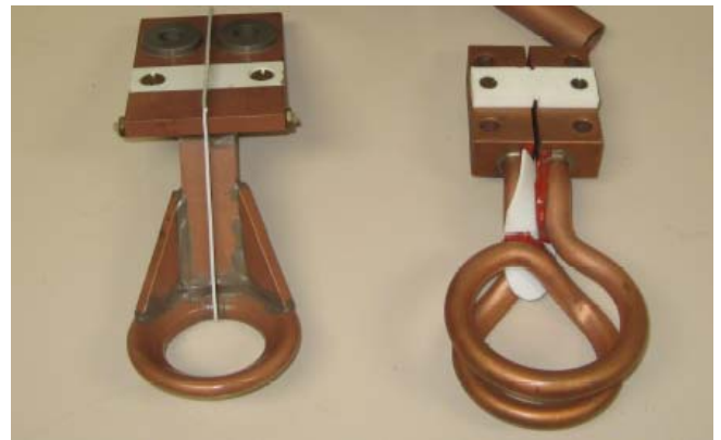
Fig.2. Single-turn and two-turn “standard” coils
