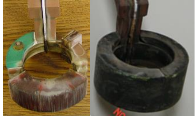
Figure 1: An image of the original production coil (left) and the redesigned coil (right) after manufacturing lifetime
