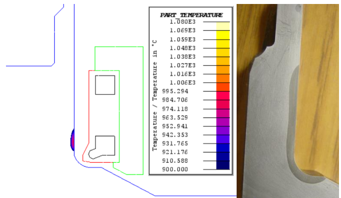
Figure 8: Comparison of redesigned coil temperatures in the wheel hub to the heat treatment pattern from a cut part
